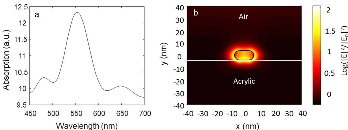
**Fig. 3.** (a) FDTD simulation of the absorption spectrum of an AuNP on an acrylic substrate. (b) The electrical field distribution was calculated at a cross section of the AuNP. At the LSPR resonance (near 550 nm), the local electrical field ( $E_0$ ) showed a 90-fold enhancement relative to that of the excitation alone. (For interpretation of the references to color in this figure, the reader is referred to the web version of this article.)
