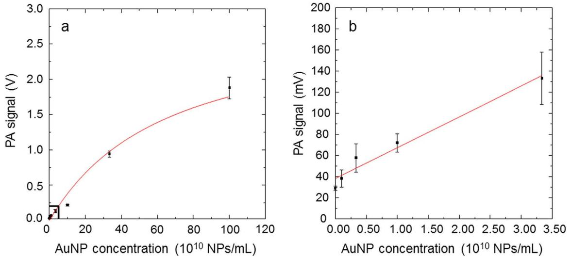
**Fig. 4.** PA signal plotted as a function of the AuNP concentration. (a) PA signals of samples at high concentrations. The PA signal approaches saturation when the AuNP concentration was increased to  $1.00 \times 10^{12}$  NPs/mL. (b) PA signals of samples at low concentrations denoted by the box in (a). The PA signal showed a linear relation with respect to the AuNP concentration. The PA signal of the acrylic substrate was 30 mV.
