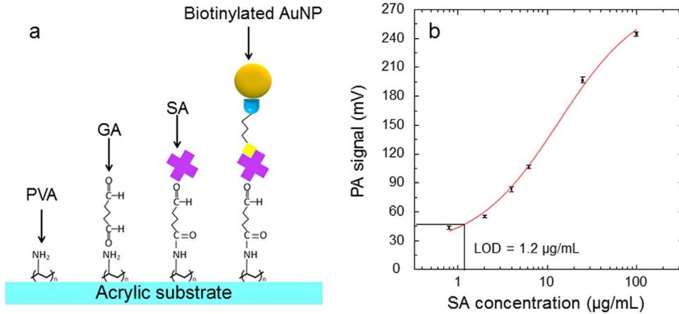
**Fig. 5.** (a) Schematic representation of the SA-measurement assay. SA was immobilized on an acrylic substrate pre-treated with PVA and GA, after which it was labeled with biotinylated AuNPs. (b) PA signal plotted against the SA concentration. The LOD was measured as 1.2 µg/mL.
